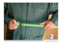
At the end of the heating period fitting and pipe end are separated from the heating elements.
