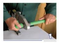
The pipe end and the socket of fitting are pushed heaters in axial direction. Pipe and fitting should be heated simultaneously.
